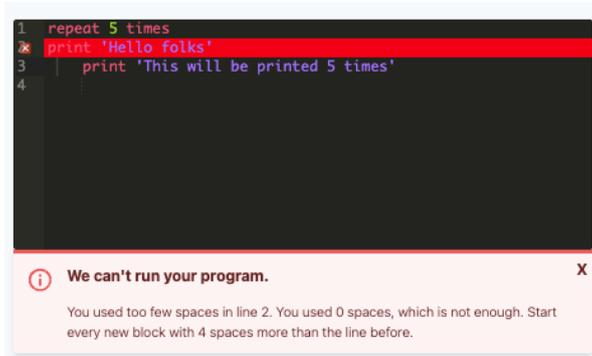
Figure 2: Error message given when indentation is missing in Level 8
