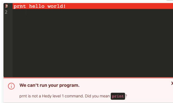
Figure 9: Misspelling a keyword in Level 1 produces an error message that is relatively easy to understand.
